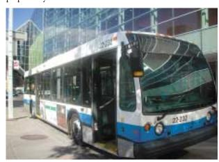
addition of touch-sensitive bars to facilitate the opening of the rear doors; increased sound-proofing, smoother acceleration; better heating and ventilation; the addition of ABS brakes; increased space in the area for wheelchairs; adjustment in the suspension to reduce the rolling sensation and a less slippery floor covering. Employees, for their part, worked on a daily basis to continue to improve these vehicles.
